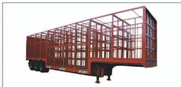
40Ft 3Axles Storehouse Semi-Trailer (Concave Beam Type)
