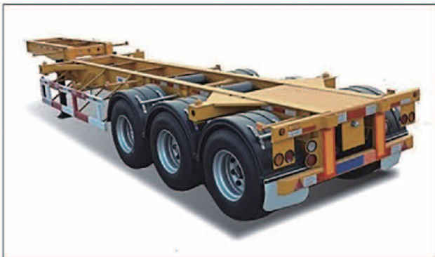
20Ft 3Axles Big Gooseneck Type Skeletal Semi-Trailer
