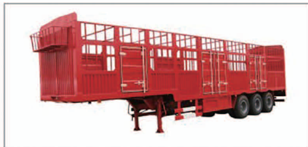
40Ft 3Axles Storehouse Semi-Trailer (Gooseneck Type)
