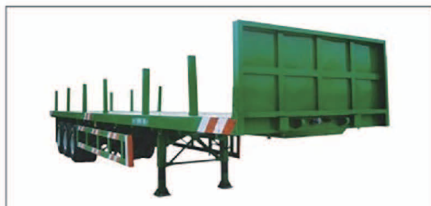
40Ft 3Axles Flatbed Semi-Trailer (With Front Wall and Stand Column)
