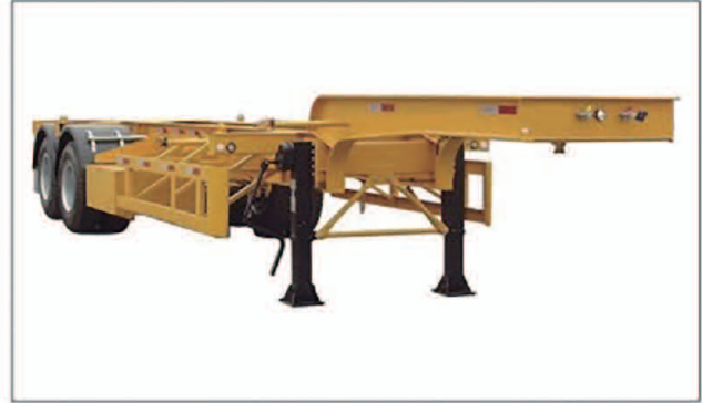
20Ft 2Axles Big Gooseneck Type Skeletal Semi-Trailer
